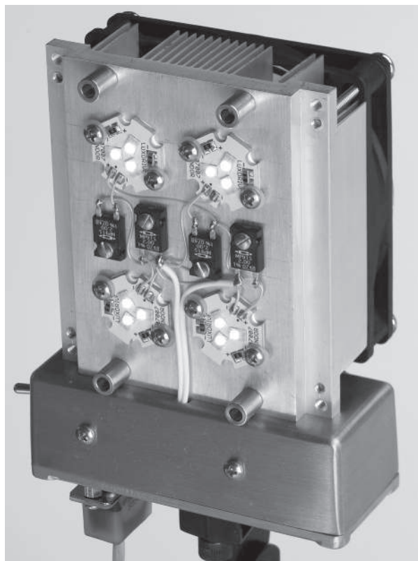
Figure 12.64. Computer CPU heatsink hijacked to make cool desk lamp. We cranked down the current so you can see the four sets of LED triples, along with the surface-mount ballasting resistors. At full brightness (1000 lumens) you can't look at this thing! The switching driver circuitry of Figure 12.63 lives in the box at bottom.
